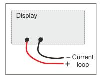
The open strand ends of the wire for connecting the current loop display are at the back of the display.
