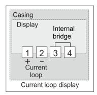
The 4-pole plug-in terminal strip for connecting the current loop display is located on the backside of the display and is only accessible after the casing is opened.
