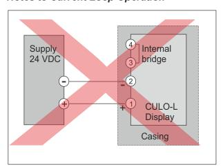
The display can only operate in a current loop of 4...20 mA.
