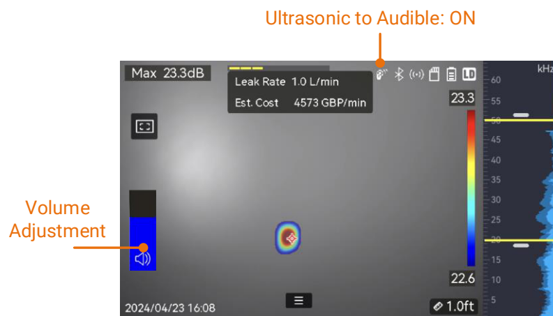
Figure 5-4 Ultrasonic to Audible and Volume Adjustment
