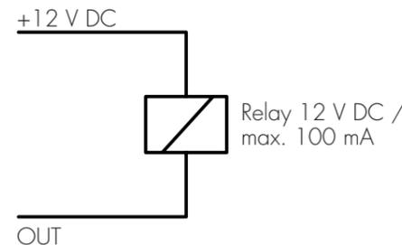
Figure 4 Example of a relay connection
