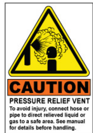
Fig. 4: Warning sticker found near the rupture disc on all meters
