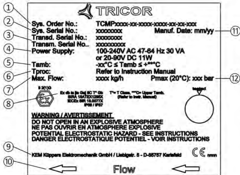
Fig. 43: TCMP system identification nameplate
