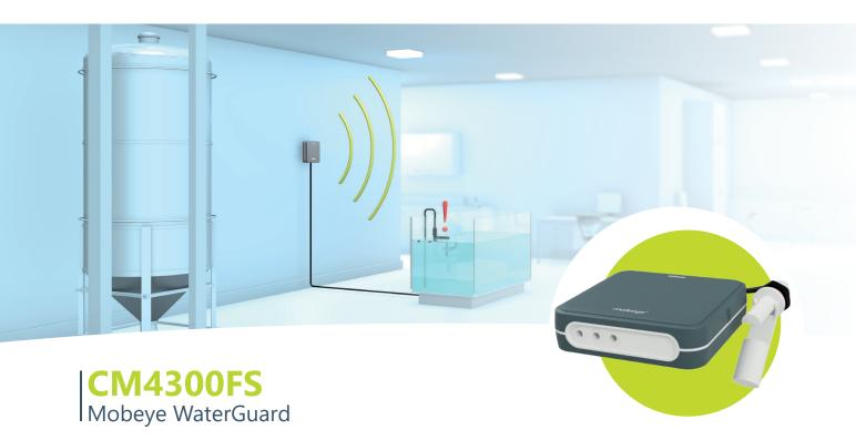
The Mobeye WaterGuard-FS informs contacts when the water level rises or falls. The device consists of a water float sensor and a compact communication box. By fixing the sensor in a horizontal position at the critical water level, it will be closed (when the water rises) or opened (when the water level falls). This is followed by an alarm message. The device is fully battery powered, or uses external power. The built-in communication module can connect to the 4G LTE-M and the 2G network.
