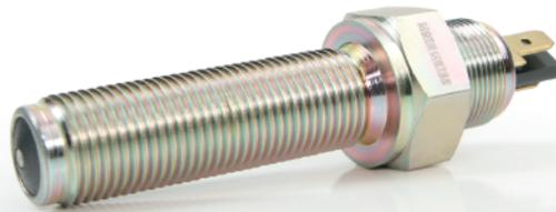
Inductive sensors are used in vehicles and machines to measure the revolutions per minute of rotating shafts, axles or wheels. The number of teeth of a toothed pulley or the holes of a holed pulley are counted by induction. The produced pulses will be transmitted to a revolution counter which will show the revolutions per minute taking into account the pulses per revolution.
