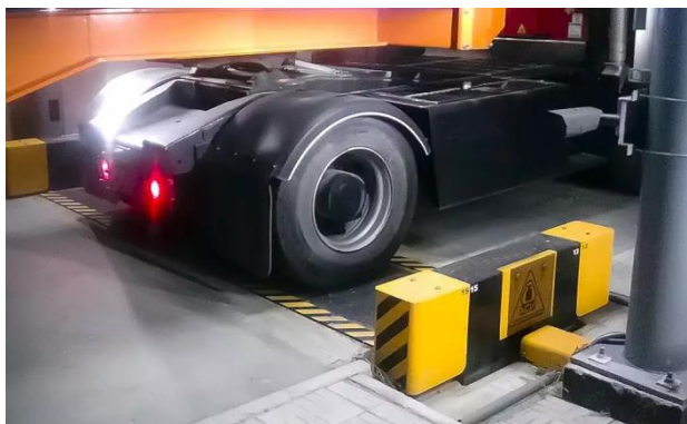
a) for weighing a single Vehicle axle
