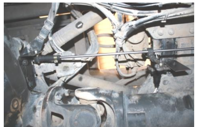
b) fixing the sensor to the frame with spot welding
