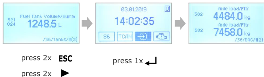
Figure 47 — Navigation keys and examples of switching between MasterCAN Display 35 G information screens
