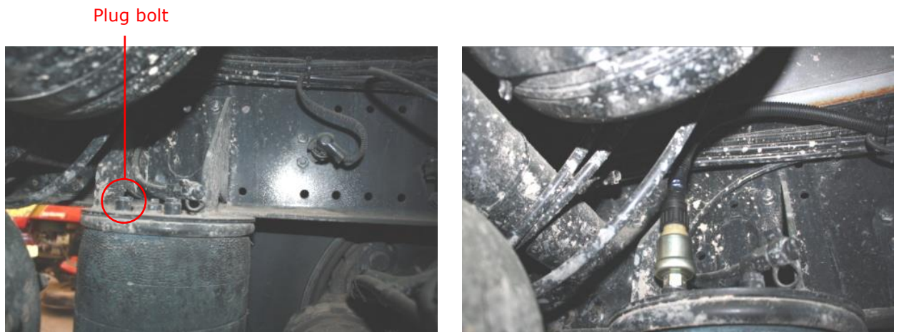
Figure 25 — GNOM DDE mounted into suspension air balloon
