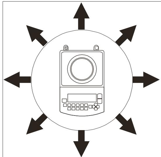
Location for the scale should be chosen with care in order to limit influence of the factors that can interrupt working scale. This location has to maintain proper temperature for working scale and necessary space for its operating. The scale should stay on stable table made of material that does not influence magnetically on the scale.
