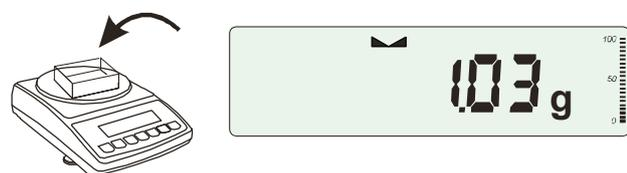
After putting container (package) tare the scale using →T← key. NET indicator will show up.
