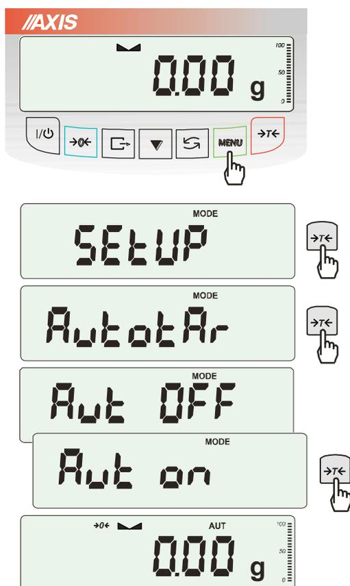
When the function is activated, the scale automatically ensures stable zero indication if the pan is empty or if zero indication was acquired by pressing →T← key.
