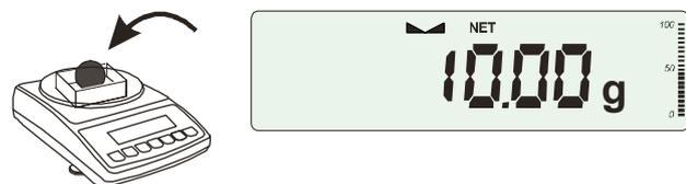
In order to readout gross weight press ↻ key (B/G indicator shows that scale indicates gross weight). Press again ↻ key in order to come back to net indications.
