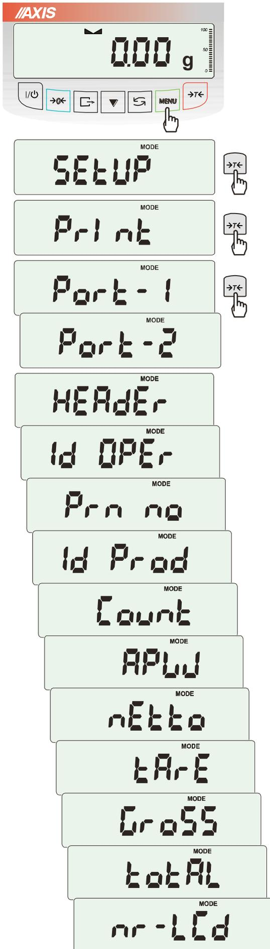
Function is used for printing additional information stored in scale memory, weighed product identification data and scale operator id. That information is inscribed using scale keys or scanner.
