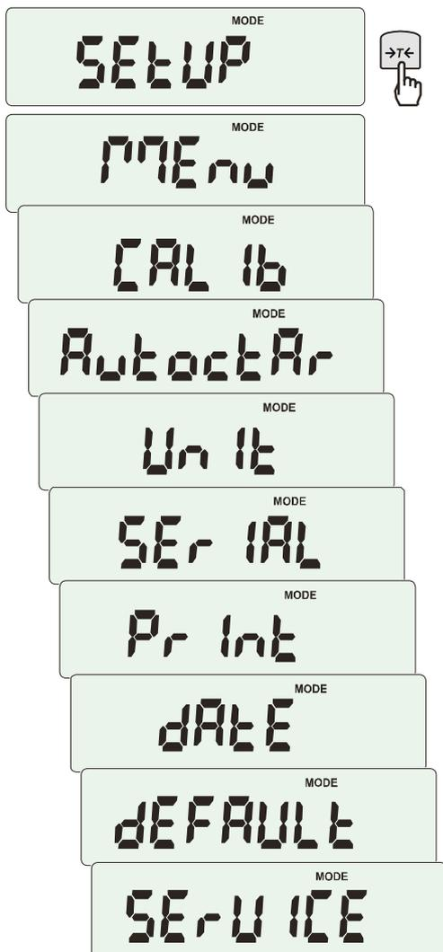
*SEtUP* contains all options used for setting scale work mode:
