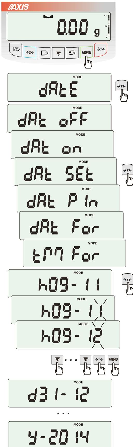
The function allows setting current date and time of scale internal clock and mode of its use.
