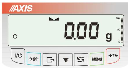
Wait until the weighing result is averaged – scale display blinks. Then scale will show stable (averaged) result and will send it through serial port.
