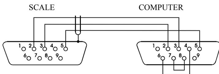
**Connecting cable WD-1 (connects printer with scale):**
