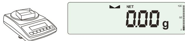
Put on weighted object and readout net weight (NET indicator shows that scale indicates net weight).
