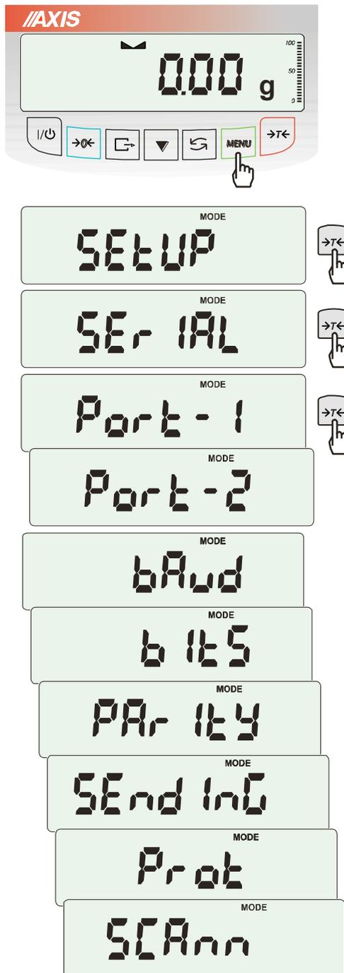
The function allows setting independently communication parameters of both of serial ports *Port-1* and *Port-2* (executed in RS232C, RS485, USB or LAN standard):
