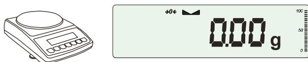
Zero indication and →0← indicator mean that the scale is ready to work.
