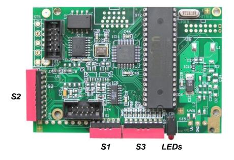
Profibus Address, internal Profibus Bus Termination (S2)
