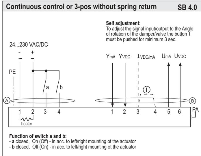
**Wiring diagram ExMax-5.10-YF and ExMax-15-YF**
