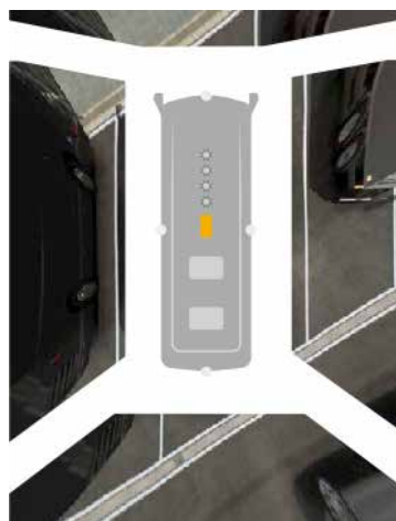
3_ The transmitted images are adjusted perspectively and consolidated to create a preview
