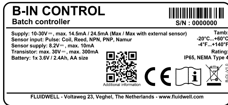
Fig. 17: External label with general data.
