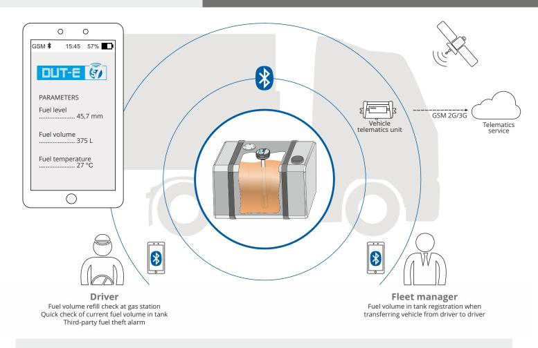
DUT-E S7 transmits data on fuel level/volume simultaneously to several devices: telematics unit, smartphones, tablets.
