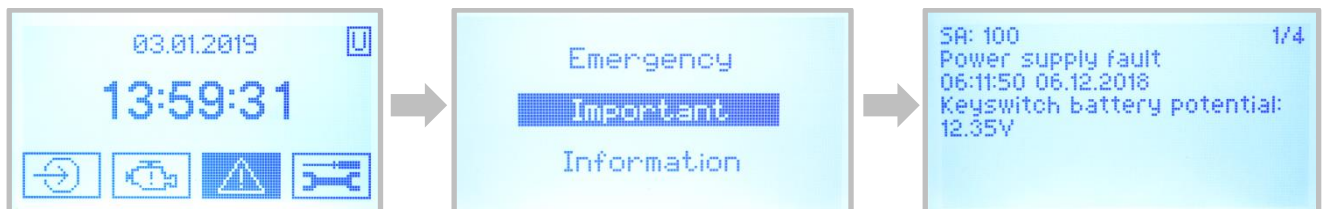
Figure 23 — Example of data display by MasterCAN Display 35 information screen containing data of an important Event from an external Unit
