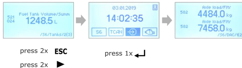
Figure 20 — Navigation keys description and examples of navigation between screens of MasterCAN Display 35
