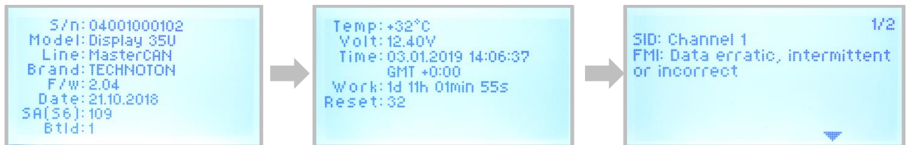
Figure 22 — Example of displaying service information screens by MasterCAN Display 35
