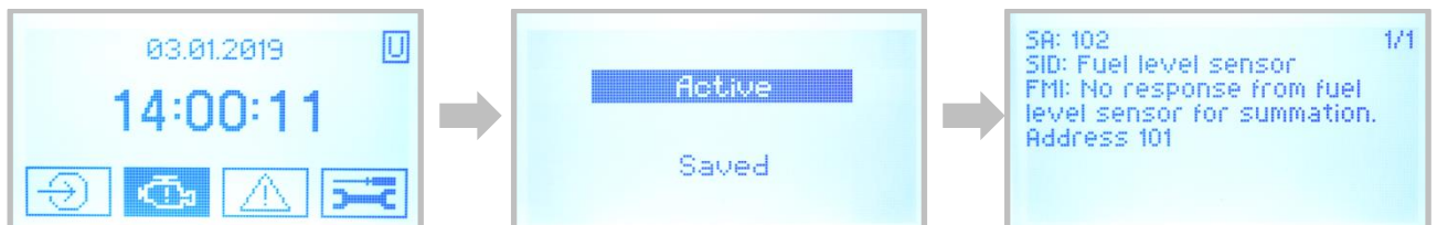
Figure 21 — Example of MasterCAN Display 35 information screen displaying data of external Unit active malfunction
