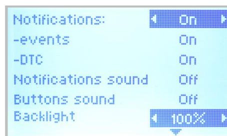
Figure 19 — View of MasterCAN Display 35 screen of settings
