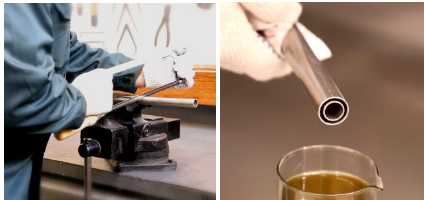
Figure 14 – DUT-E measuring probe cutting
