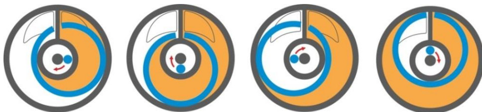
Figure 9 – DFM Marine measuring chamber operation scheme
