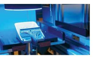
The SF, gas density controllers are set individually and tested for accuracy.
