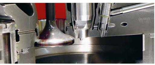
To ensure that the large engines used in ships and generators meet the strict environmental requirements and emission standards, precise and long-term stable sensors are needed for monitoring and controlling the injection pressure of over 2000 bar.
