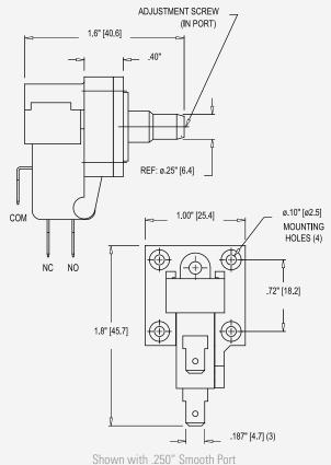
The versatile high-current PSF109S vacuum switch offers a controllable hysteresis (deadband); a wide-range field adjustable set point; snap action; and choice of standard vacuum port design options. For custom applications, our in-house design and engineering team provide rapid prototyping and manufacturing turnaround.
