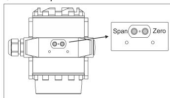
Below the product label there are 2 keys for easy configuration of zero and span. The keys are Hall effect devices and are completely seperated from other parts of the casing.
