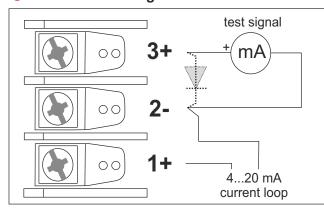
The 4...20 mA test can be measured without interruption of the low-potential circuit between terminal 3(+) and terminal 2(-). The output current is measured with an ammeter for mA across a diode in the output circuit.
