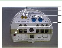
rotary switch for fail-safe mode rotary switch for probe length
