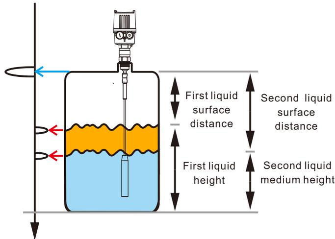
Dual Liquid Level Interface Measuring Condition:
