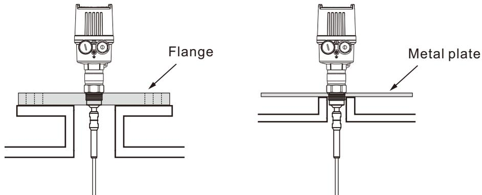
During installation, please avoid using the extension tube on the container. Please install the sensor leveled with the top cover of the container as possible. If this cannot be done, please use a shorter extension tube. Please do not install this instrument at the inlet to ensure that the meter is in a stable position in the medium and not in the inflow position of the liquid to avoid false measurements when the liquid flows in.
