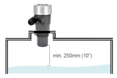
These are examples of common **INCORRECT** mountings which can prevent the unit from operating correctly.
