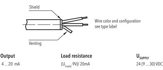
Shield in the device is not connected.
